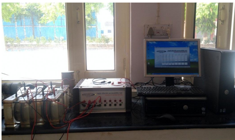
Figure 3.6 : Rapid Chloride-ion Permeability Test
