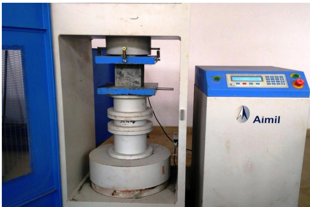
Figure 3.3 : Compressive Strength Test on Compression Testing Machine
