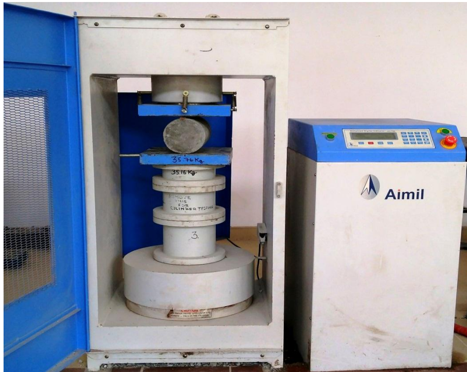
Fig. 3.4 : Splitting Tensile Strength Test of Concrete
