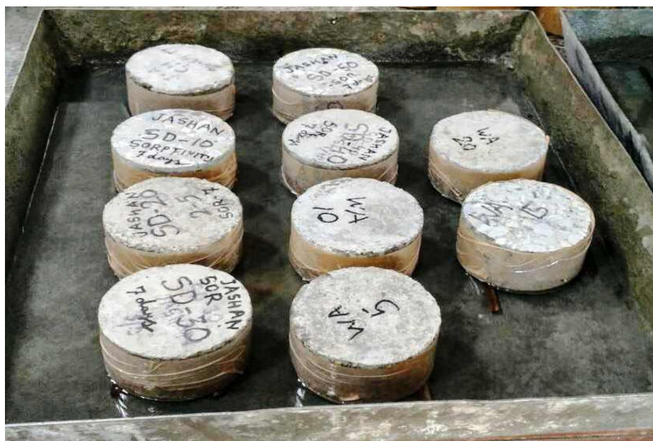
Figure 3.5 : Sorptivity Test of Concrete Samples
